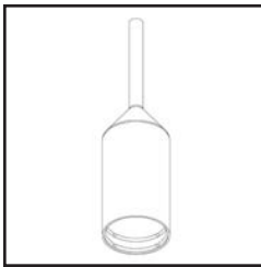
PDM 8218 Ø 6.50" with Ø 1.10 cable exit, 28.00" overall.
